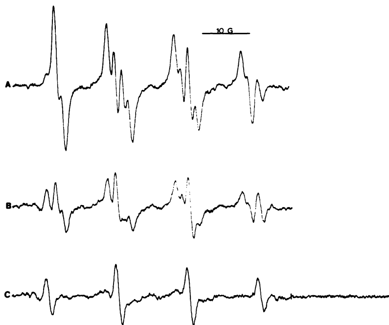
FIG. 2. Electron paramagnetic resonance spectra obtained 30 seconds, 3 min, and 12 min after the addition of tetramethylammonium superoxide/DMF solution to 50 mM pH 7.8 chelexed phosphate buffer containing 0.18 M DMPO and 1 mM DETAPAC
