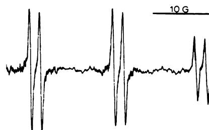
FIG. 9. Epr spectrum formed by reaction of \text{O}_2 with 4-POBN in a system consisting of 75 nM xanthine oxidase, 400 \mu\text{M} xanthine, 1 mM DETAPAC, 20 mg/ml 4-POBN, in 50 mM pH 7.8 chelexed phosphate buffer
